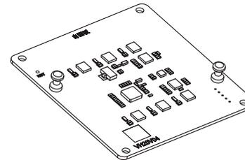
When you need to perform self-test and diagnosis on the device interface, you can take off the magnetic shield, remove the VH13 interface adapter board and insert the VH20 self-test board. Run the software help/ZIF48 self-test menu to complete the self-test.
