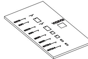
As shown in the above figure, the 6-pin, 8-pin and 16-pin chips are soldered on the adapter board which can be used to read and write the related chips.
