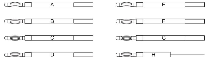
In order to connect various different types of ECUs, the device has 8 different types of ECU cable plugs, and the corresponding plugs can be selected to connect the ECU pins.
