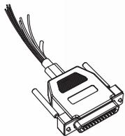
Plug the cable into the DB44 port of the device, read and write ECU module data according to the wiring diagram.
